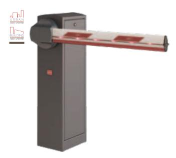
Range of professional 230 Vac electromechanical barriers for busy use, designed and developed to operate in a wide variety of conditions such as large parking lots, motorway toll-gates with frequent reversing, sensitive sites where the bar must open spontaneously in case of a power failure and in industrial installations. Mechanical movement with crank to make the bar operate smoothly, also managing slowdowns in opening and closing.
